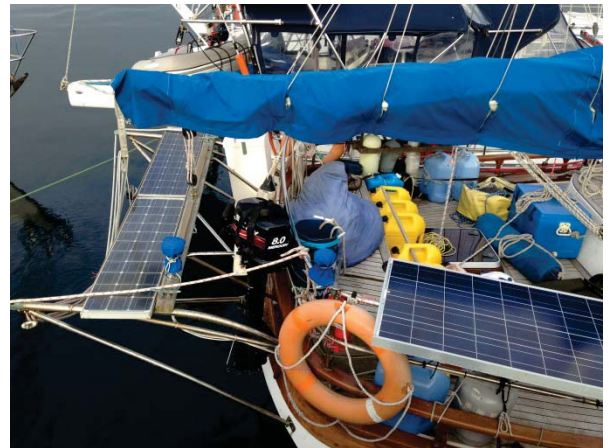
Solar panels provide everyday power to this sail boat
